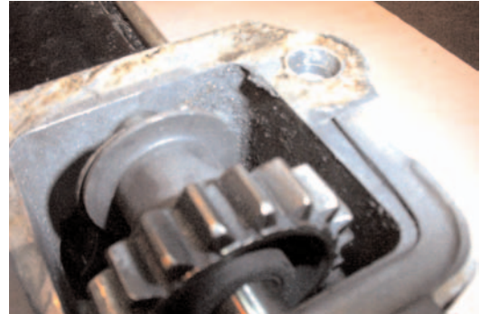
Fig.1 Fine metal particles from Dual Mass Flywheel, clutch dust contamination of the pinion and drive assembly.
